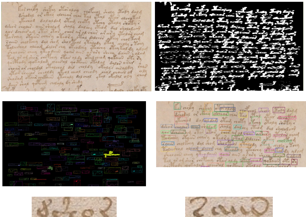
Figure 5. Image processing steps in detecting words. A. Part of source image B. Binarized and dilated image. C.1., C.2. Identified contours and bounding rectangles D. Two of the identified words
